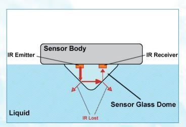
The sensor contains an infrared-ray emitter and an optical receiver. In air (liquid not present), all the light emitted is reflected — internally — by the dome and then redirected to the receiver. When the liquid reaches the sensor dome, a big amount of the light emitted is lost in the liquid and the sensor senses its presence.
